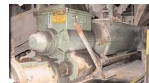
(2) Bonnot Pug Mills w/Vacuum Compressor
