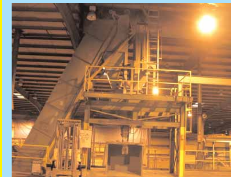
Kato 40' Skip Hoist Elevator w/Mixer, Reactor, Dust Collector
