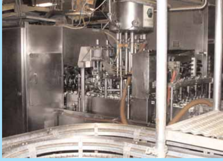
(10) FILLING LINES including Evergreen N7 Small Sections Filler
