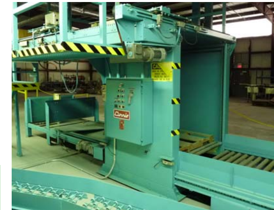
Currie Palletizer with GE PLC Controls
