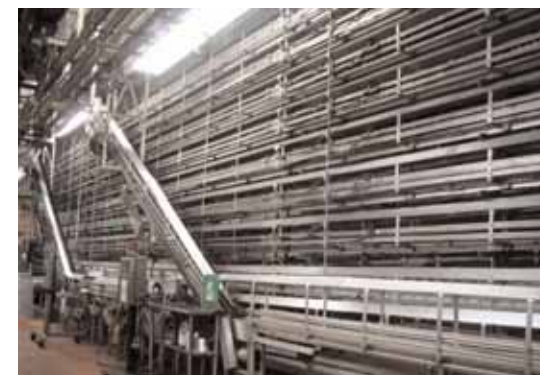
Over 3,200 ft. of Gallon and Half-Gallon Jug Conveyor
