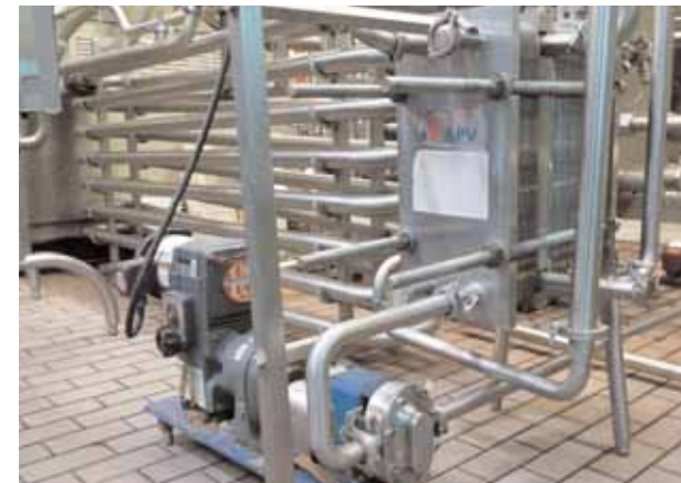
APV Cream HTST System w/Plate Press
