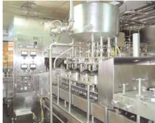
Evergreen Half-Gallon Filler w/2003 Fitment Spout/Cap System
