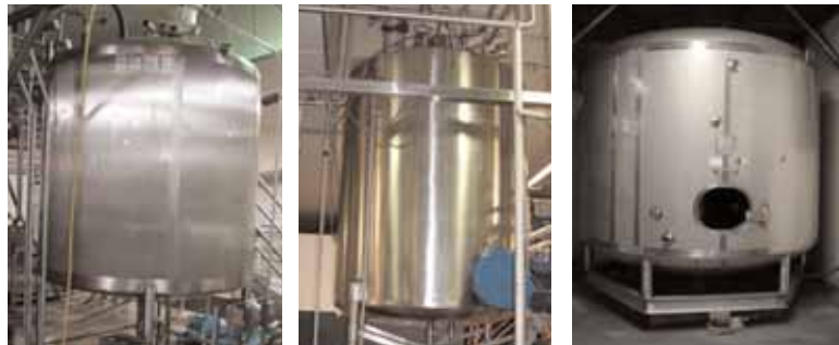
APV, Metalcraft & Walker 2,000-3,000 Gal. S/S Blend Tanks
