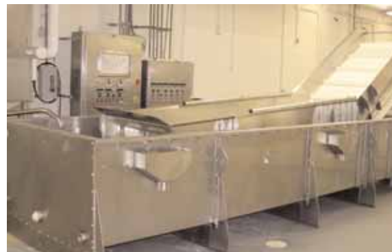
Chill Tank & Chiller System (see below)
