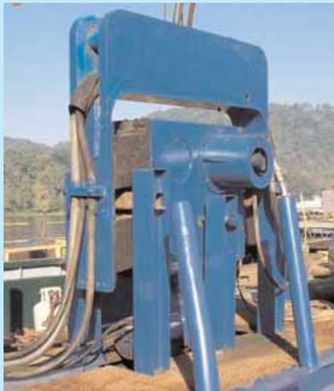
Vulcan 2800 Vibratory Pile Hammer - "Ozark" 400 hp Towboat - Spud Barge w/200-Ton 50' A-Frame
