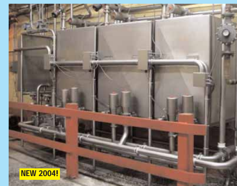
2004 Ecolab 3-Tank Skid Mounted CIP System
