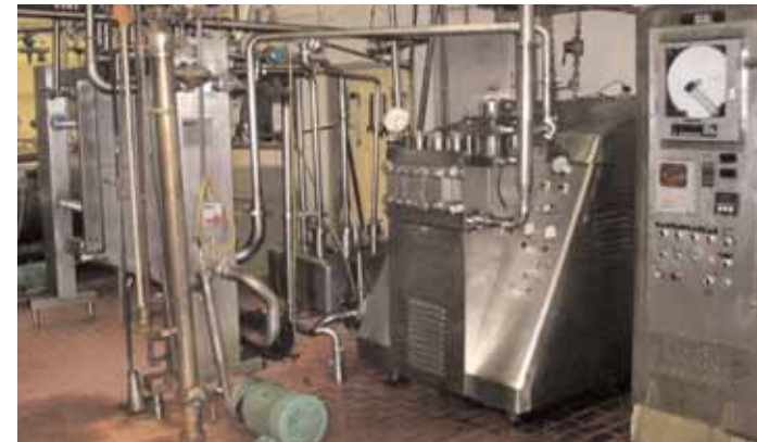
APV 5,000 gph HTST System & Manton Gaulin MC45 Homogenizer
