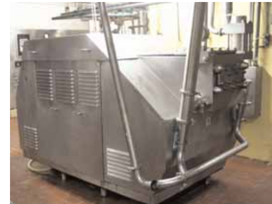
Manton Gaulin Model 804 Homogenizer
