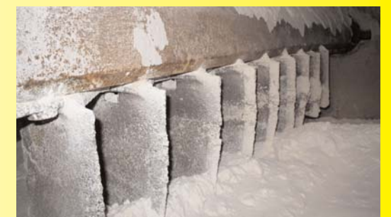
Furnace Teeth and Arms with High Nickel Content
