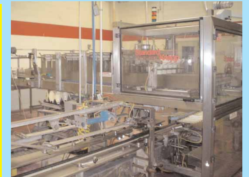
1996 Standard Knapp Type 939 S/S Case Packer
