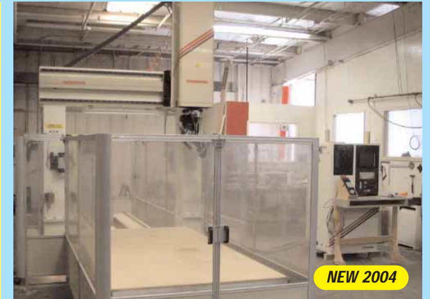
2004 Thermwood CNC Laser Calibrated Wood Router
