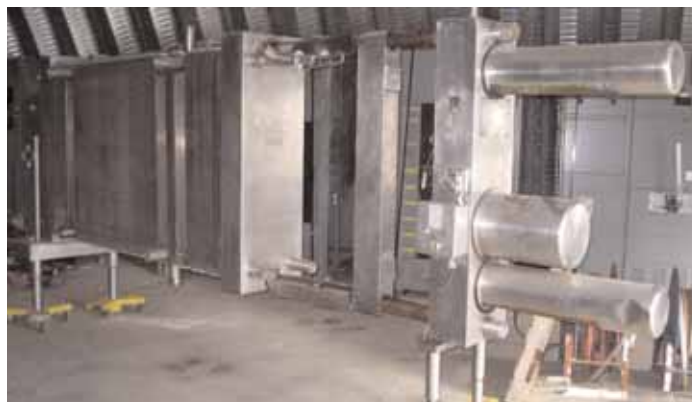
DeLaval P45-RC S/S Plate Press w/Hydraulic Open & Close
