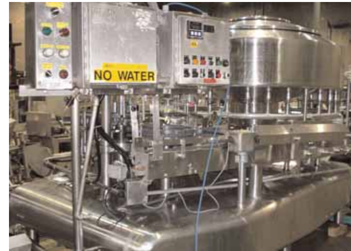
Federal 36-Valve PET Bottle Filler with 12-Head Capper and Federal 30-Valve Filler with 10-Head Capper
