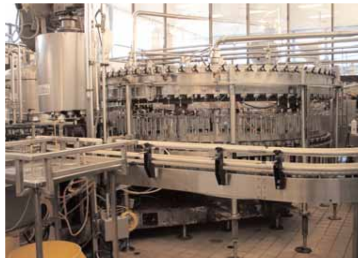
HK 72-Valve Rotary Filler & Fowler/Zalkin Capper
