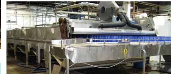
Above: I & H Cooling Tunnel
