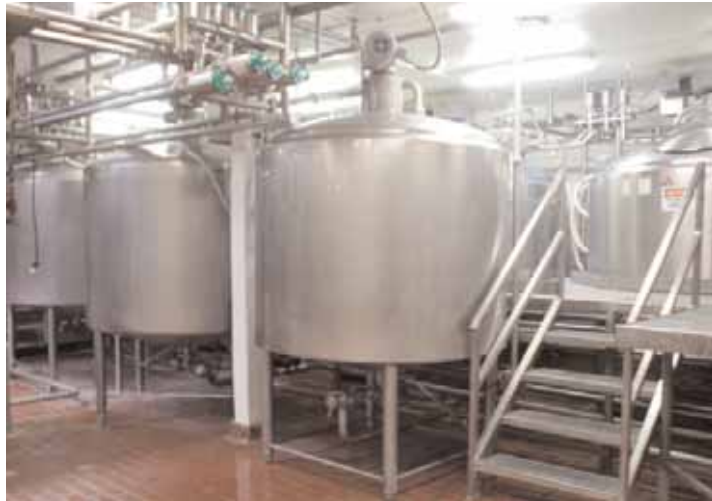
(15) APV Crepaco & other S/S Processors including Dome-Top, Cone-Bottom Processors
