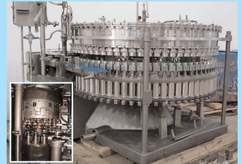
Meyer 72-Valve Rotary Filler and Sasib 10-Head Seamer (Inset)
