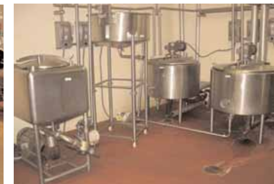
Pilot Plant: (3) 50 Gal. Mix Vats, 50 Gal. Liquifier
